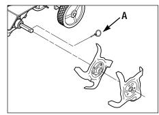
Figure 16: Remove ring lock pin (A) to take off tines.
